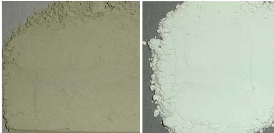
FIGURE 12. GRAY TYPE I-II PORTLAND CEMENT (LEFT) (ALBEDO 0.32) AND WHITE TYPE I PORTLAND CEMENT (RIGHT) (ALBEDO 0.87) (LEVINSON, 2001).
