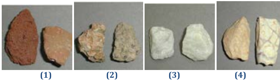
FIGURE 11. LIGHT COLORED ROCK AGGREGATE: (1) DARK RED VOLCANIC ROCK (BASALT) (ALBEDO 0.17), (2) BLACK AND RED ROCK (GRANITE) (ALBEDO 0.19), (3) WHITE ROCK (PLAGIOCLASE) (ALBEDO 0.49), AND (4) GOLD AND WHITE ROCK (CHERT, IRON IMPURITIES) (ALBEDO 0.55) (LEVINSON, 2001).
